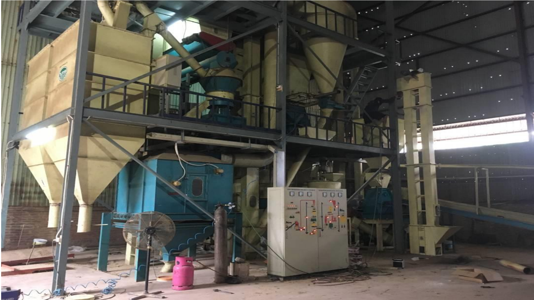
Equipment for processing pellet feed for cattle - capacity of 800 - 1,000 kg / h
