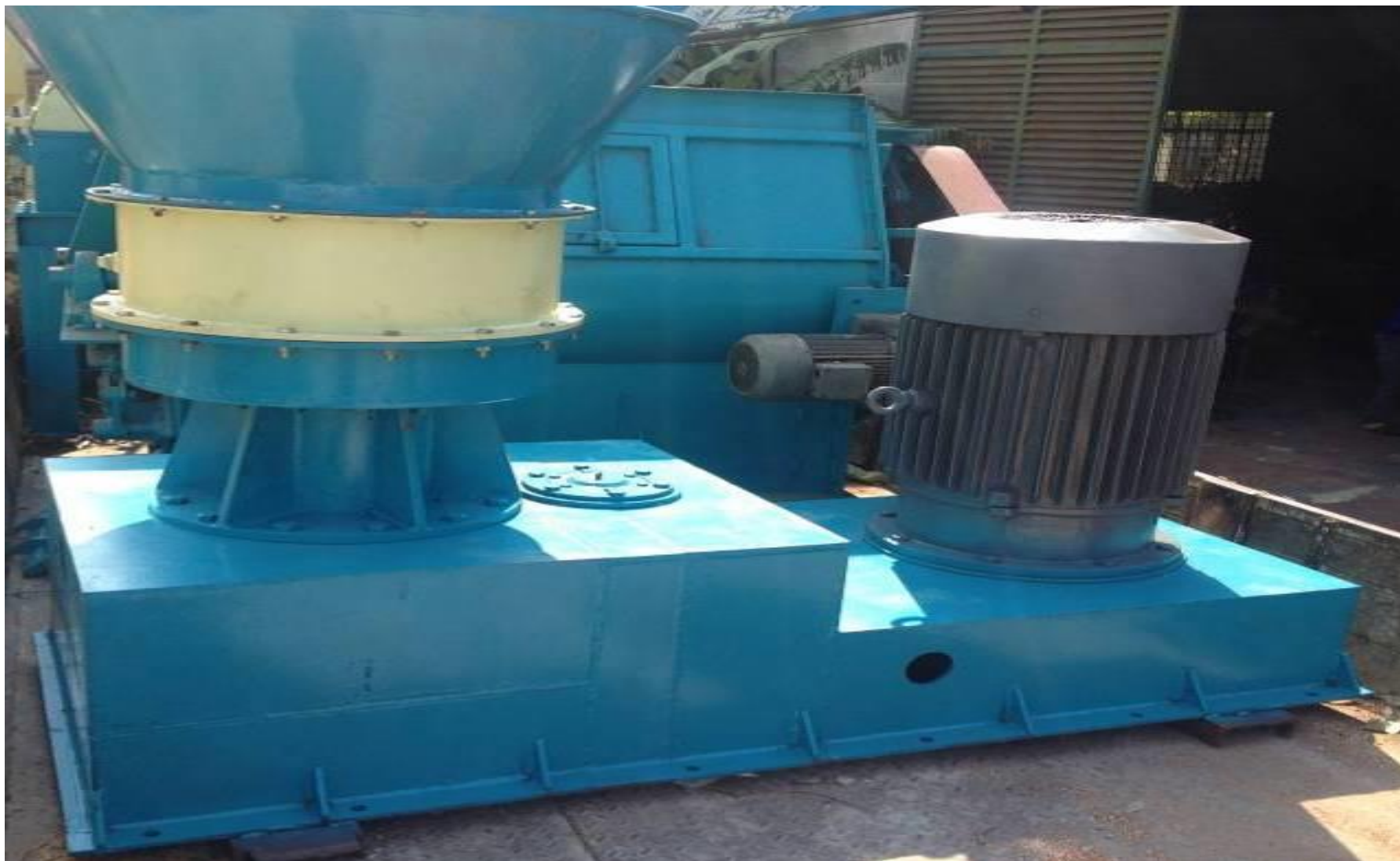
Pelleting machine, capacity 800 - 1,000 kg / h
